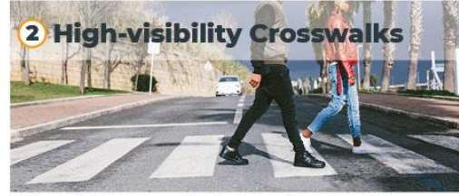
2 High-visibility Crosswalks High-visibility crosswalks that are aligned as close as possible to the pedestrian clear path and minimally setback from the intersection puts the pedestrian into the drivers field of vision.
